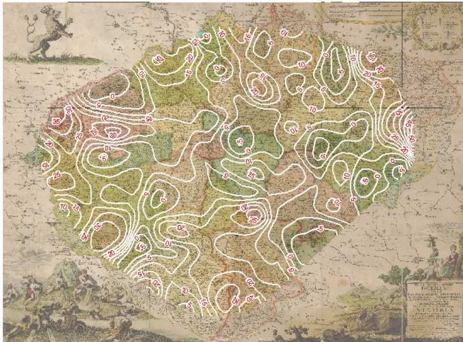
Figure 5: Rotation isolines of Vogt's map generated with the step 10^\circ .
